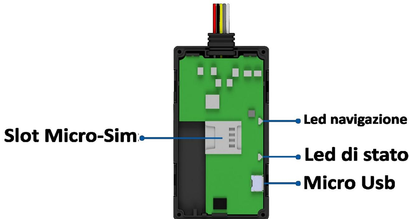
Figure 1 FMB920 device view
